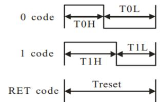
**Example:** The information required from WS2812B datasheet is the Data Transfer Time as below:
