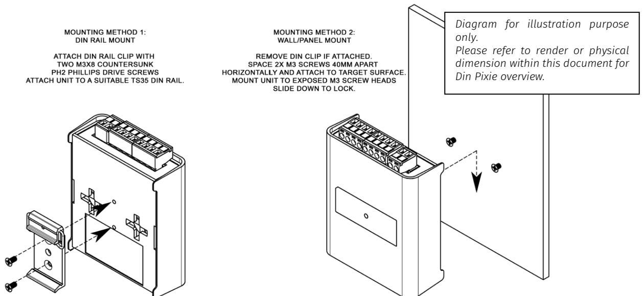
**Note:** The surface mount tabs have been designed to hold the weight of the DIN PIXIE only, excess force caused by cable strain can cause damage.
