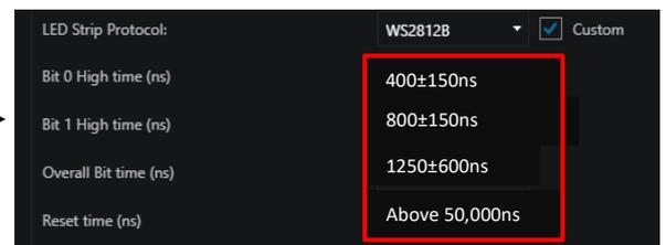
\* Please test on your pixel fixture for the optimal transmission time among the range according to the datasheet.
