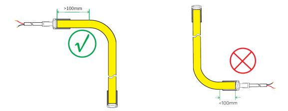
Ensure that the feeding cable does not bear any force and allow for a 10mm lead with a loose configuration. This will help prevent any strain or stress on the cable, ensuring optimal performance and longevity.
