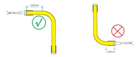
• Ensure that the feeding cable does not bear any force and allow for a 10mm lead with a loose configuration. This will help prevent any strain or stress on the cable, ensuring optimal performance and longevity.
