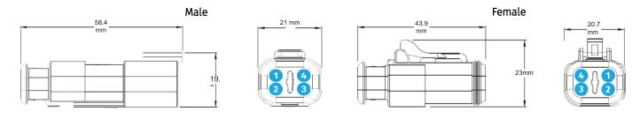
All ENTTEC Smart PXL Dot accessories feature premium IP-rated automotive-style connectors with an integrated latching system. Cables and connectors are reinforced with industrial-grade heat shrink for enhanced durability and long-term reliability. View each accessory's datasheet for more information.
