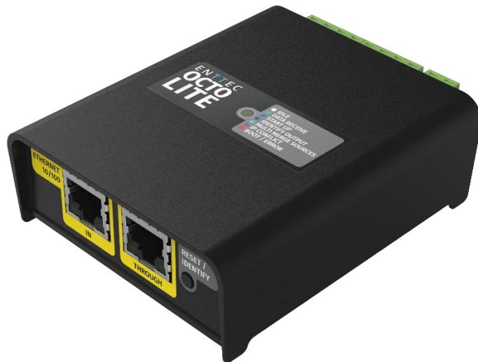
The ENTTEC OCTO LITE is a compact, and DIN-rail-compatible 8U pixel controller engineered for immediate Ethernet-to-SPI conversion. It efficiently processes up to 8 universes of Art-Net, sACN, and ESP over Ethernet, delivering 4 universes per output supporting LED fixtures with clock line.
