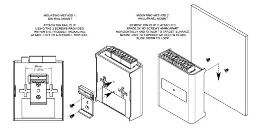
**Note:** The surface mount tabs have been designed to hold the weight of the OCTO MK2 only, excess force by cable strain can cause damage.
