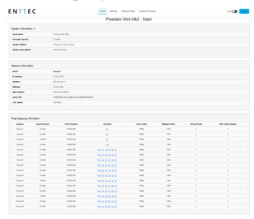
Select the Universe number to reveal the current DMX buffer. This can be manually refreshed to capture a frame snapshot or set to auto-refresh to view channels in real time. Up to 2 Universe buffers on separate ports can be revealed at once.
