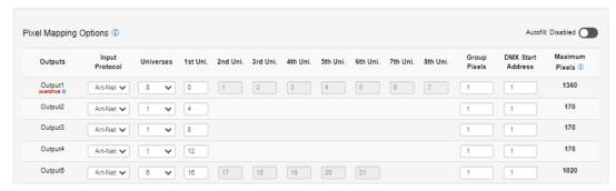
It allows the option of using the same universes for all outputs. Alternatively, each output can be configured to use unique set of universes. For example, output 1 can use universes 100, 101, 102, and 103, while output 2 uses universes 1, 2, 3, and 4.
