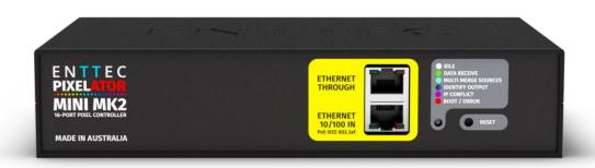
The ENTTEC PIXELATOR MINI MK2 is a high-performance 16-port Ethernet pixel controller designed for large-scale LED installations, converting up to 128 Universes of Art-Net, sACN, and ESP protocols into SPI within the PLINK system.
