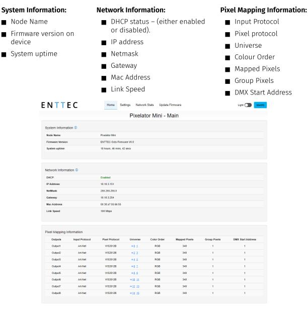
Select the Universe number to reveal the current DMX buffer. This can be manually refreshed to capture a frame snapshot or set to auto-refresh to view channels in real time. Up to 2 Universe buffers on separate ports can be revealed at once.
