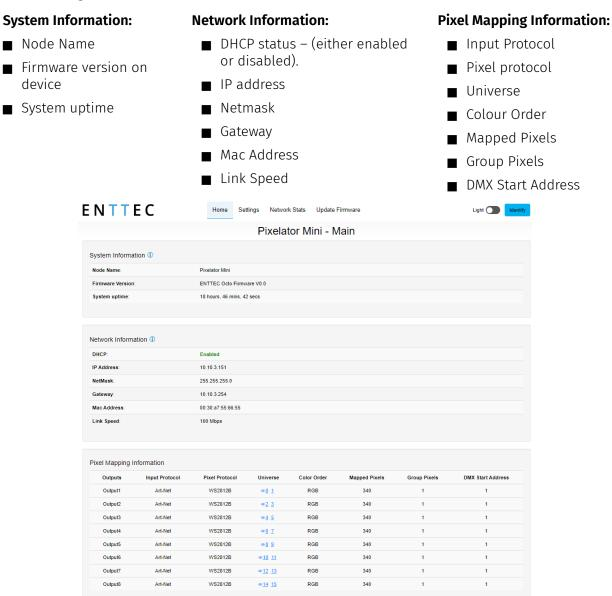
Select the Universe number to reveal the current DMX buffer. This can be manually refreshed to capture a frame snapshot or set to auto-refresh to view channels in real time. Up to 2 Universe buffers on separate ports can be revealed at once.
