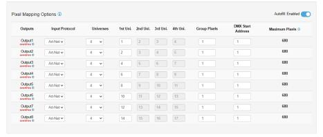
It allows the option of using the same universes for all outputs. Alternatively, each output can be configured to use unique set of universes. For example, output 1 can use universes 100, 101, 102, and 103, while output 2 uses universes 1, 2, 3, and 4.
