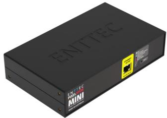
The ENTTEC PIXELATOR MINI MK2 is a high-performance 8-port Ethernet pixel controller designed for large-scale LED installations, converting up to 32 Universes of Art-Net, sACN, and ESP protocols into SPI within the PLINK ecosystem.
